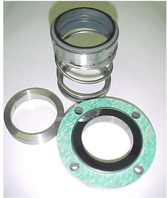
New Carbon Seal Face, New Bellows Rubber Ultra-sonic Clean all SS Parts New SS Set-screws in Drive Collar New Tungsten Carbide Seat with Slot Install New SS Pin in Gland Plate Manufacture New Gland Plate Gasket
