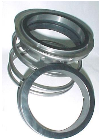
New Tungsten Carbide Rotary Face New Rubber Bellows Clean, Lap & Polish Tungsten Carbide Seat
